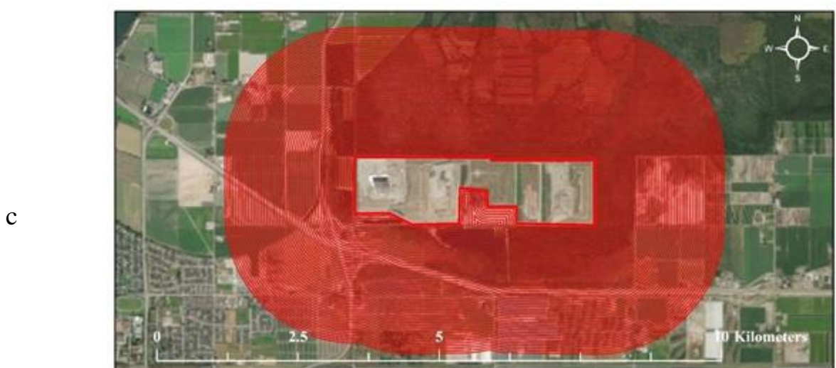
657 Supplementary Figure 1 - Vancouver landfill. (a) Layout of Vancouver landfill including active, capped and future 658 phases (Source: Vancouver, 2017), (b) digitizing the actual boundaries of landfill using Arc-GIS10.5 software, (c) 659 Construction of multiple ring buffer zone with 30-meter increments around the landfill for up to 1500 meters 660
